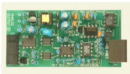
Analog output board for scaled 0-20 mA or 4-20 mA plus 0-10 Vdc analog outputs.
